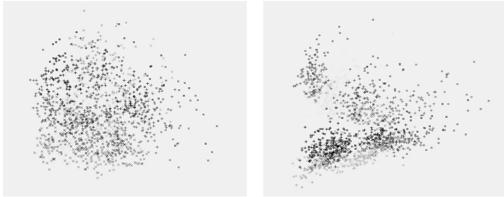
Figure I.4: A simple example of exploratory projection pursuit. On the left, a random 2-D projection of the 4-D data set of vowel formant frequencies due to (Peterson and Barney, 1952). On the right, a 2-D projection of the same data set that has been optimized by exploratory projection pursuit, using the Friedman-Tukey projection index.
