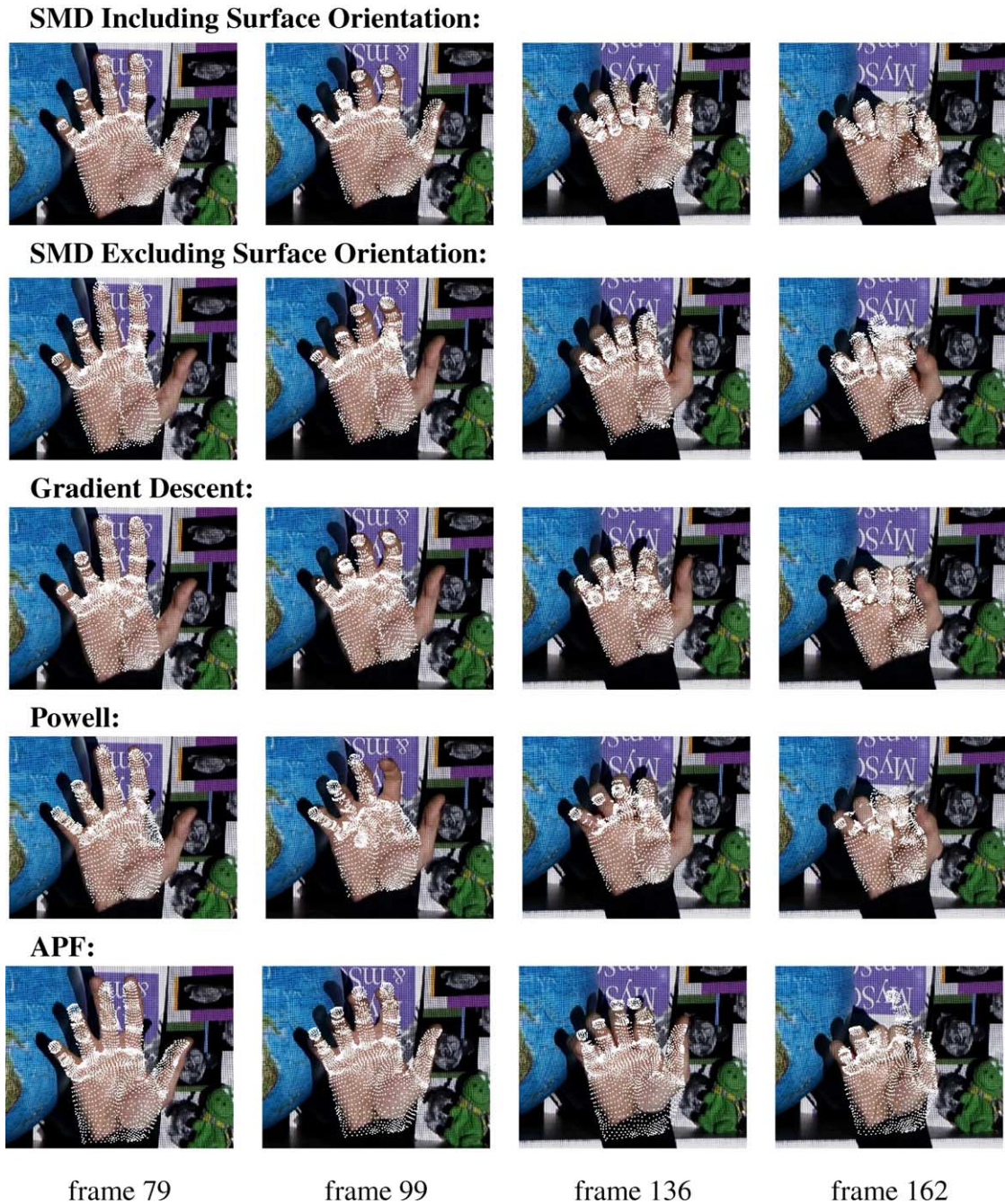
Fig. 10. Comparison between SMD and alternative optimization algorithms. From top to bottom: the results of the SMD using a cost function E evaluating the distances and the differences in surface orientations, SMD using a cost function E only evaluating the distances, gradient descent, Powell and annealed particle filter (APF). The model is visualized as the vertices of the skin polygonal representation. The pictures have been cropped for better visibility, but see Fig. 11 for examples of similar, complete frames.
