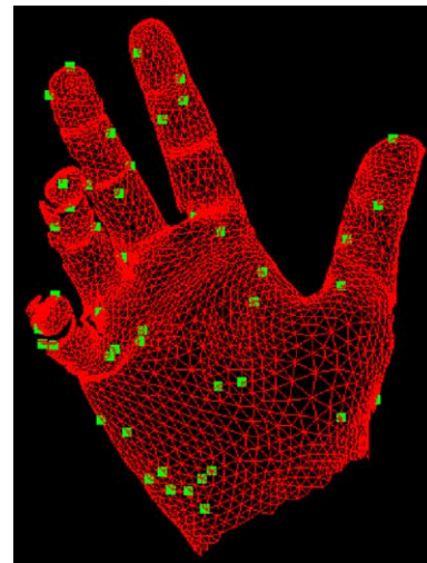
Fig. 5. On the left (a), evolution of the tracker's speed according to the number of sample points and the sampling mode. On the right (b), illustration of a random subsampling performed on the hand model with 2 points per phalanx and 15 points for the visible part of the palm. When a hand part is not visible, the points expected on it are randomly chosen on any other visible part.
